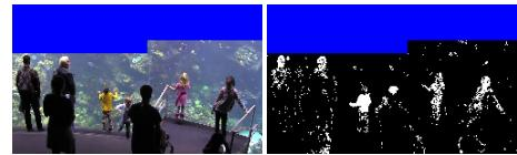
**Figure 14:** Left: we apply a mask, shown in blue, on the surveillance video to restrict and accelerate the detection. Right: relative background subtraction result; white regions are with motion.
