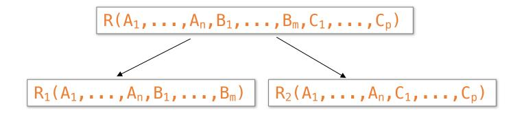
A decomposition R to (R1, R2) is <u>lossless</u> if R = R1 Join R2
